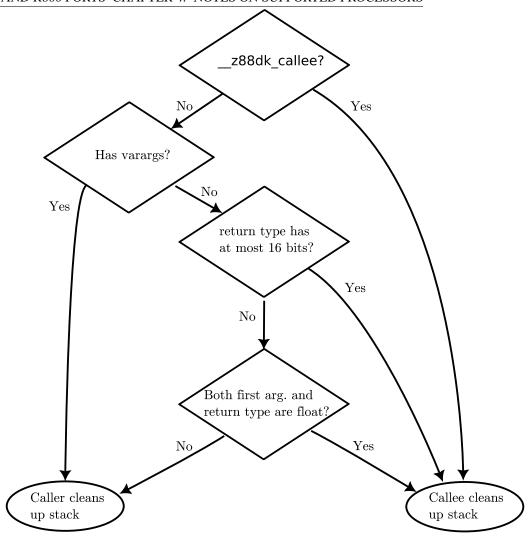
If \_\_z88dk\_callee is not used, after the call, the stack parameters are cleaned up by the caller, with the following exceptions: functions that do not have variable arguments and return void or a type of at most 16 bits, or have both a first parameter of type float and a return value of type float.
