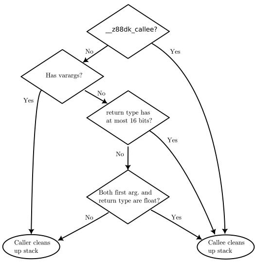
If \_\_z88dk\_callee is not used, after the call, the stack parameters are cleaned up by the caller, with the following exceptions: functions that do not have variable arguments and return void or a type of at most 16 bits, or have both a first parameter of type float and a return value of type float.
